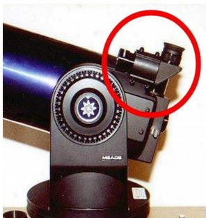
is a small telescope of weak magnification providing a broad image of the sky and displays cross-hairs at the eyepiece image. Some guidescopes come with a 90° prism or mirrored eyepiece to provide more comfortable viewing during observations.
